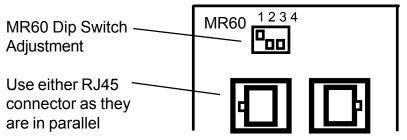
The rear of the MR60 is shown. Because one to three MR60's can be connected or daisy chained to the same cat 5 wire, the keypad position on the wire must be selected using the dip switch. The two MR60 RJ45 connectors are in parallel. Only one dip switch slider should be on and the other two off (#1 is shown on in this example). The MR60 1-2-3 dip switch positions correspond to MVP64 keypad ports and speaker outputs A1-A2-A3 or B1-B2-B3.
